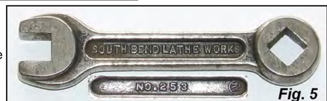
Fig. 5. 4 inch spanner with square O/E and socket embossed, (obverse) SOUTH BEND LATHE WORKS, and (inverse) No.253 and RI, in a roundel. - Rhode Island Tool Company according to Alloy Artefacts
