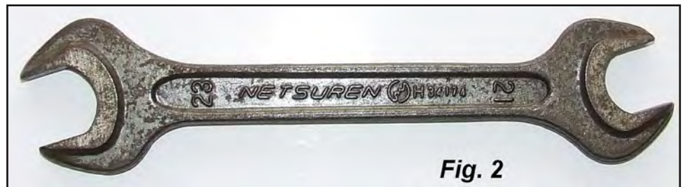
Fig. 2. 220mm O/E spanner embossed (-obverse panel) 23 NETSUREN (trademark) 23 H34174 21, and (inverse panel) JIS B 4630 21x23.
