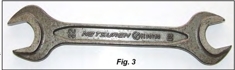
Fig. 3. 275mm O/E spanner embossed (-obverse panel 32 NETSUREN (trademark) H 35160 30, and (-inverse panel) M22 JIS B 4630 30x32 M20.
