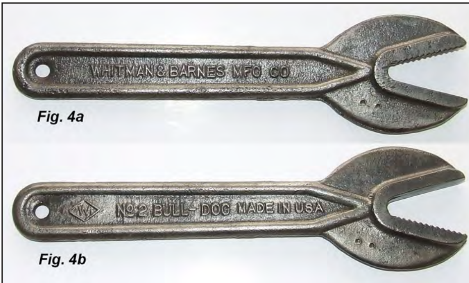
Fig. 4a & 4b. both sides of a 9 inch alligator wrench (1 1/2 inch jaw (max.) embossed
