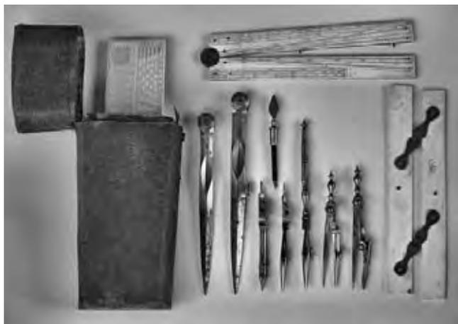
*Illus 3 – A set of drawing instruments from about 1800 showing a vertical fishskin case*
