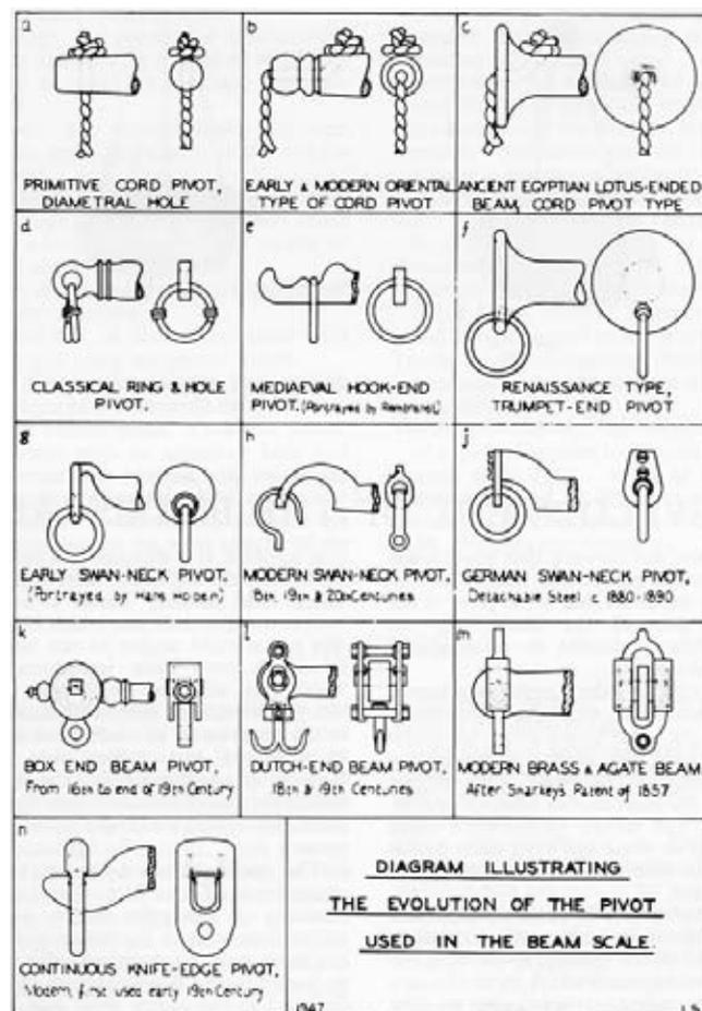
Fig. 4. Sketch of the development of balance beam ends
